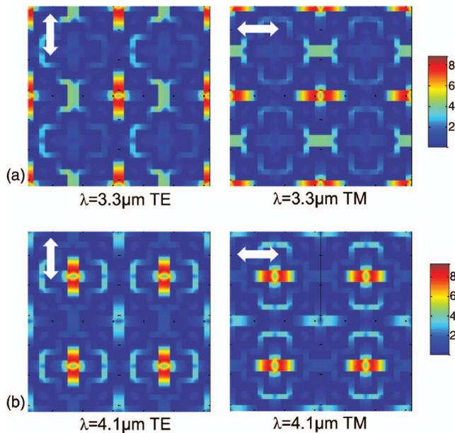
FIG. 3. (Color) The relative surface current distribution on the metal elements at the two resonance wavelengths: (a)  $3.3 \mu\text{m}$  and (b)  $4.1 \mu\text{m}$  for two orthogonal polarizations, induced at normal incidence. The white arrows indicate the polarization. The colored bars indicate the relative current density.
