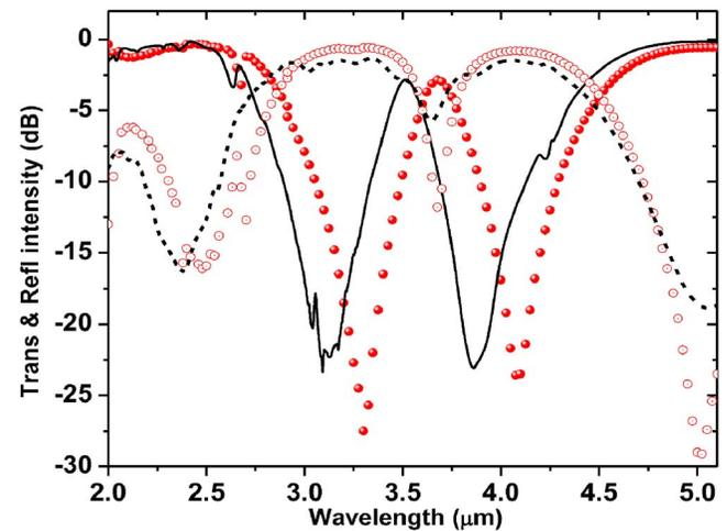
FIG. 2. (Color online) PMoM-modeled transmission spectrum (filled red circles) and reflection spectrum (empty red circles) at normal incidence of the designed metallodielectric filter shown in Fig. 1(a). Measured transmission spectrum at normal incidence (solid black line) and reflection spectrum at 15° (dashed black line) of the fabricated filter. Both spectra were taken using an unpolarized source.
