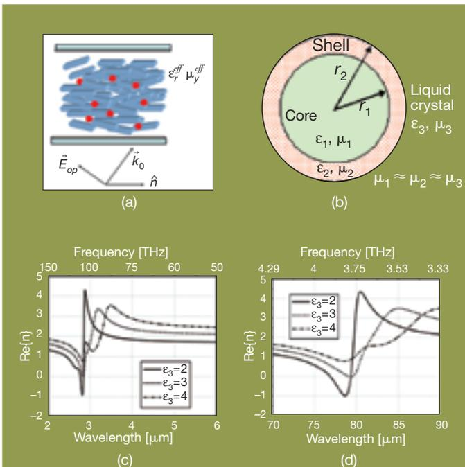
(a) A planar aligned nematic liquid crystal containing core-shell nano-spheres. (b) Cross-section of the core [ $\mu_1, \epsilon_1$ ]-shell [ $\mu_2, \epsilon_2$ ] nanosphere with the liquid crystal host [ $\mu_3, \epsilon_3$ ]. (c) Tunable refractive index of the nano-sphere dispersed liquid crystal as a function of liquid crystal host permittivity in the optical region. (d) Tunable refractive index as a function of liquid crystal host permittivity in the terahertz region.
