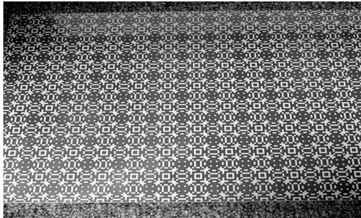
**Figure 1:** A photograph of the actual GA-designed high impedance FSS ground plane that was fabricated and tested for GPS and cellular operation.
