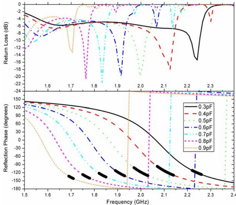
**Figure 4:** Antenna return loss and EBG surface reflection phase.
