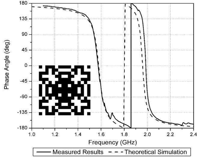
**Figure 2:** Simulated versus measured reflection coefficient phase for the dual-band GPS and cellular GA-designed high impedance FSS. The FSS unit cell geometry is shown as an inset on the reflection phase response plot.
