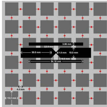
**Figure 3:** Geometry of the broadband open-sleeve dipole over a narrowband tunable EBG.
