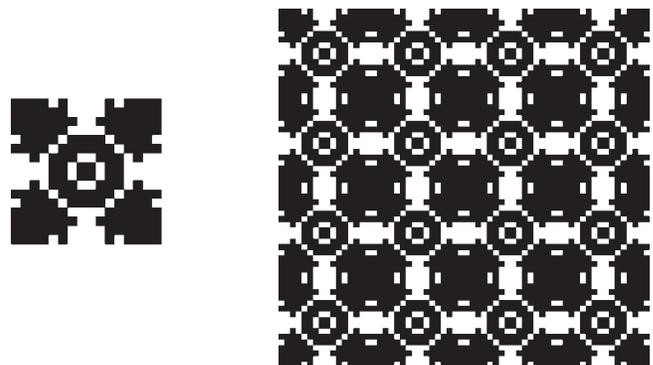
**Figure 5** Unit cell geometry and corresponding FSS screen geometry for an additional ultrathin electromagnetic bandgap absorber with magnetic substrate
