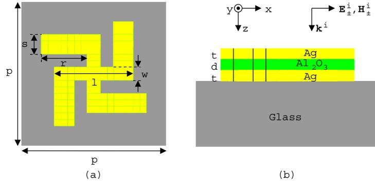
Fig. 1. The unit cell of the planar chiral metamaterial: (a) A top view, (b) A side view.
