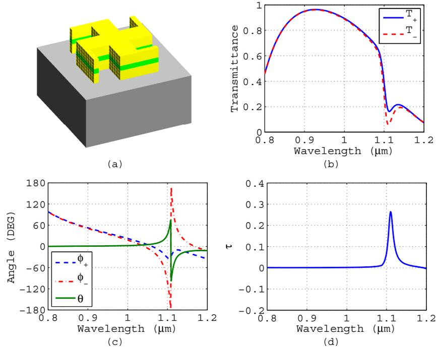
Fig. 3. An optimized metamaterial for strong polarization rotation under the condition  $T_{\min} = 0.5$ : (a) The optimized unit cell geometry, (b) the transmittances  $T_{\pm}$ , (c)  $\phi_{\pm}$  and  $\theta$ , and (d) the ellipticity  $\tau$ . The maximum rotation of  $\theta = 21^{\circ}$  is achieved at  $\lambda = 1.093 \mu\text{m}$ . The dimensions of the optimized design are listed in Table 1.
