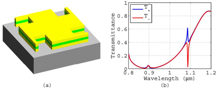
Fig. 2. An optimized metamaterial for strong CD in the near IR: (a) The optimized metamaterial geometry, (b) The transmittance responses.
