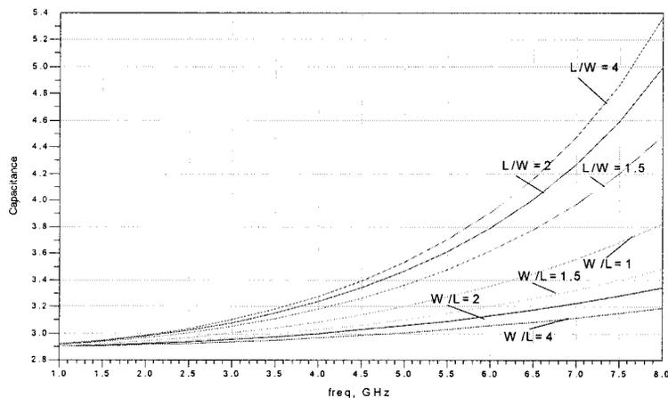
Figure 10 The capacitances of circuit model with different  $W, L$
