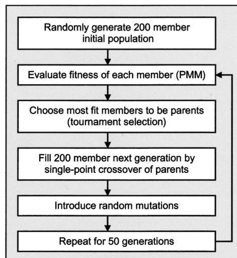
FIG. 1. Flowchart of the GA used for MDPC design.
