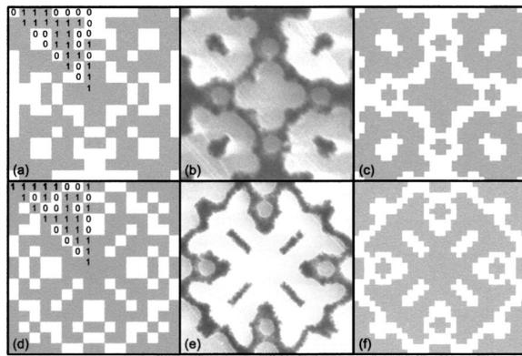
FIG. 2. (a) GA-optimized unit cell with overlaid chromosome values of the MDPC designed for a  $0.5 \mu\text{m}$  polyimide substrate with stop bands at 23 and  $43 \mu\text{m}$ . (b) SEM image of the fabricated MDPC. (c) Modeled geometry trimmed to the fabricated MDPC. (d)–(f) Corresponding process for the MDPC designed for a  $4 \mu\text{m}$  thick polyimide substrate with stop bands at 38 and  $75 \mu\text{m}$ .
