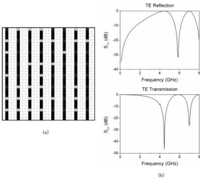
**Figure 1** (a) A dipole RFSS geometry with GA optimized switch settings “1” indicates the switch is closed and a “0” indicates the switch is open; (b) frequency response (transmission and reflection) for the FSS is shown in (a)
