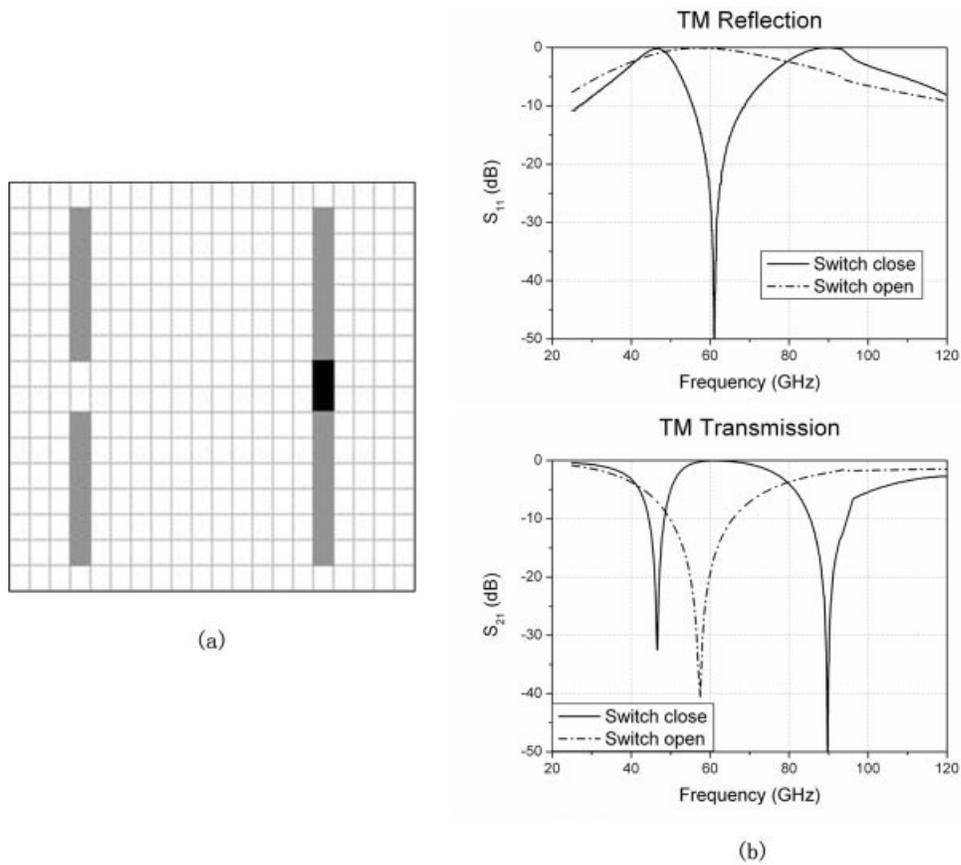
**Figure 5** (a) Unit cell (black blocks indicate the switch is closed); (b) frequency response (transmission and reflection) for the RFSS is shown in (a)
