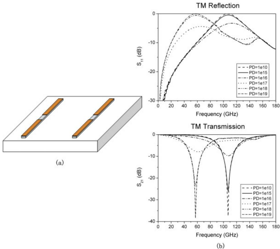
**Figure 4** (a) Unit cell of metallodielectric RFSS with silicon switches; (b) frequency response (transmission and reflection) for the RFSS is shown in (a). [Color figure can be viewed in the online issue, which is available at [www.interscience.wiley.com](http://www.interscience.wiley.com)]
