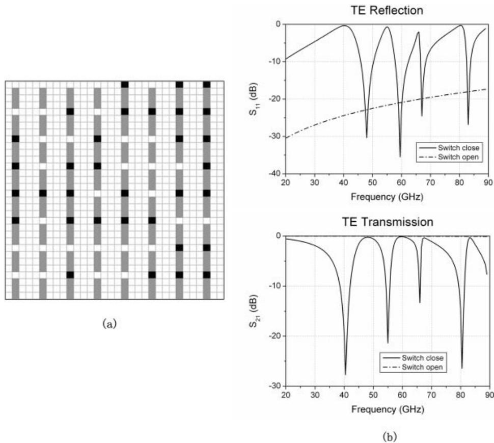
**Figure 6** (a) GA optimized unit cell geometry (black blocks indicate the switch is closed); (b) frequency response (transmission and reflection) for the RFSS is shown in (a)
