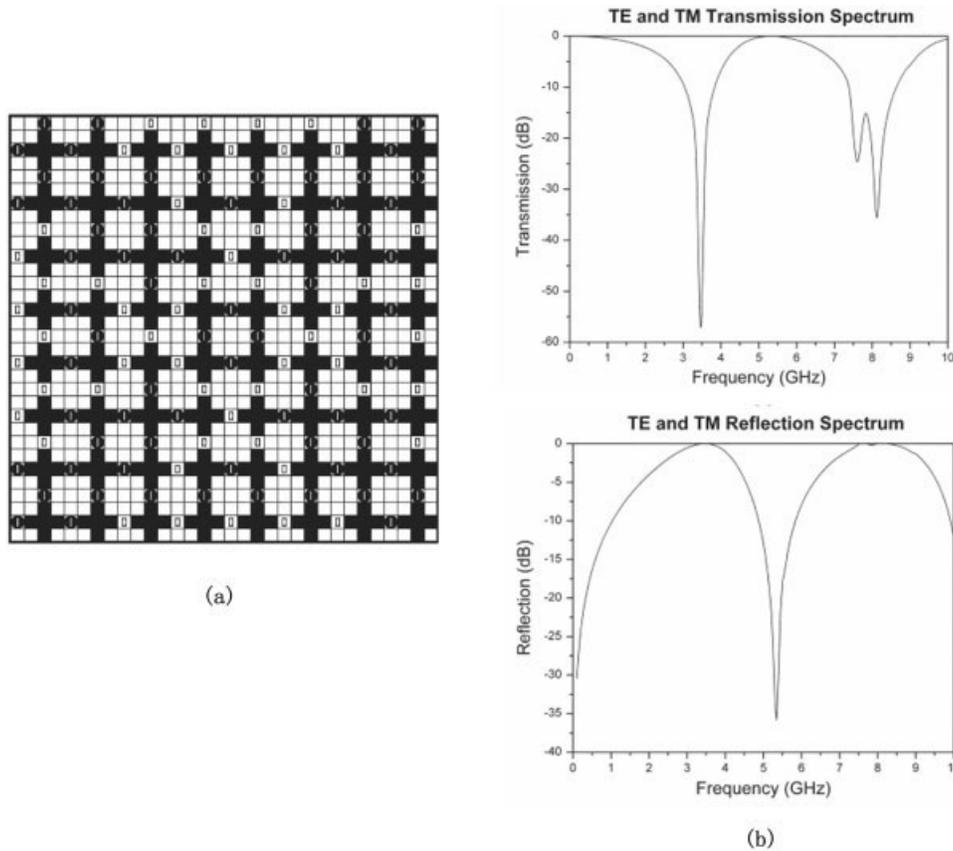
**Figure 2** (a) A cross-dipole RFSS geometry with GA optimized switch settings “1” indicates the switch is closed and a “0” indicates the switch is open; (b) frequency response (transmission and reflection) for the FSS is shown in (a)
