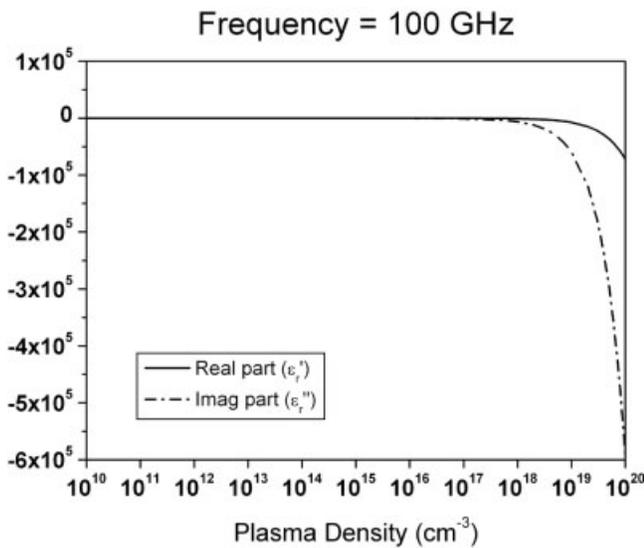
**Figure 3** Calculated permittivity of silicon under varying photonic excitation
