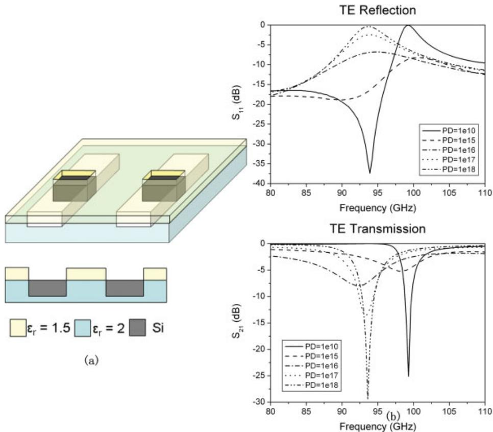
**Figure 7** (a) Unit cell and cross section of an all-dielectric RFSS; (b) frequency response (transmission and reflection) for the RFSS shown in (a). [Color figure can be viewed in the online issue, which is available at [www.interscience.wiley.com](http://www.interscience.wiley.com)]
