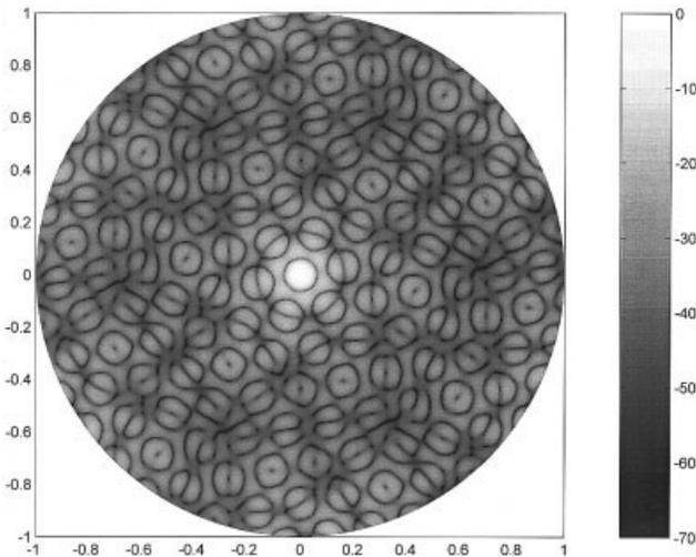
**Figure 5** Contour plot of the normalized radiation pattern for a stage-3 Peano–Gosper fractile array with 344 elements
