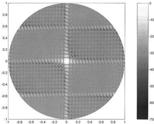
**Figure 4** Contour plot of the normalized radiation pattern for a 352-element hexagonal array
