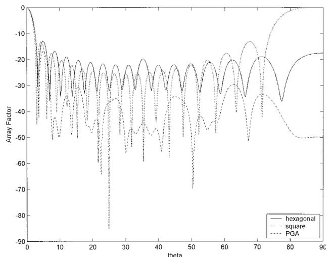
**Figure 3** Plots of the normalized array factor vs.  $\theta$  in degrees with  $\varphi = 90^\circ$  when the element spacing is  $d_{\min} = \lambda$  for a  $19 \times 19$  square array, a 352-element hexagonal array, and a 344-element stage-3 Peano-Gosper array (PGA)
