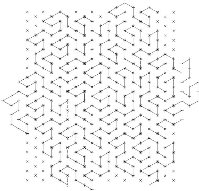
**Figure 1** Element locations for a stage-3 Peano-Gosper fractile array (344 elements) and a 352-element hexagonal array
