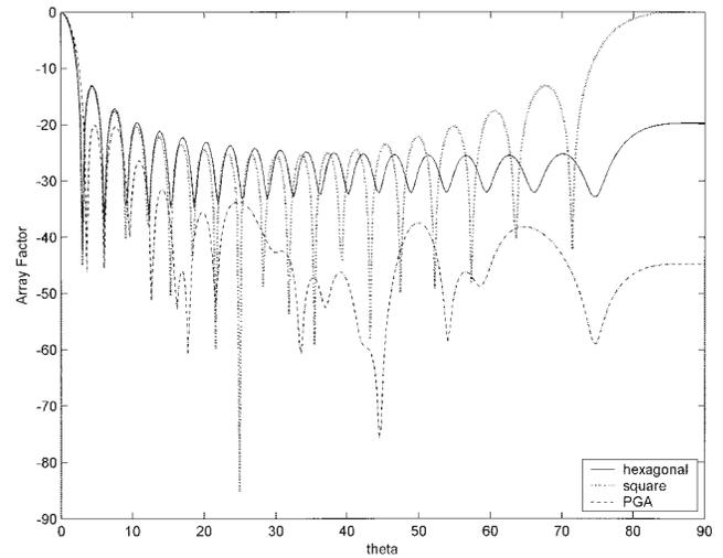
**Figure 2** Plots of the normalized array factor vs.  $\theta$  in degrees with  $\varphi = 0^\circ$  when the element spacing is  $d_{\min} = \lambda$  for a  $19 \times 19$  square array, a 352-element hexagonal array, and a 344-element stage-3 Peano-Gosper array (PGA)
