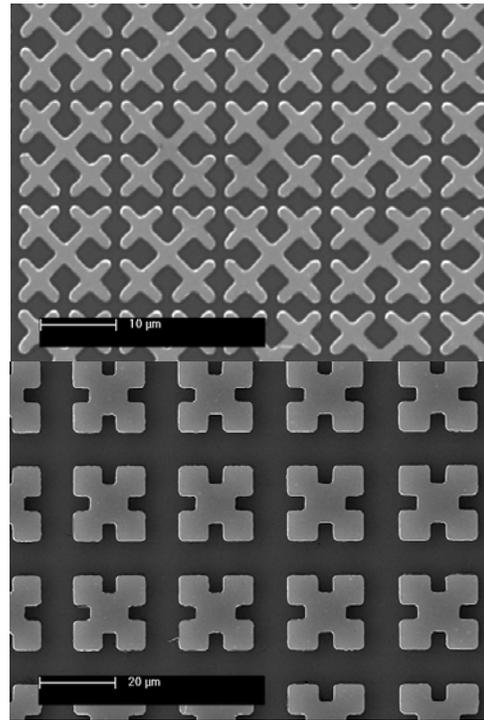
SEM images of fabricated fractal cross-dipole (top) and fractal square patch (bottom) metallic patch arrays.
