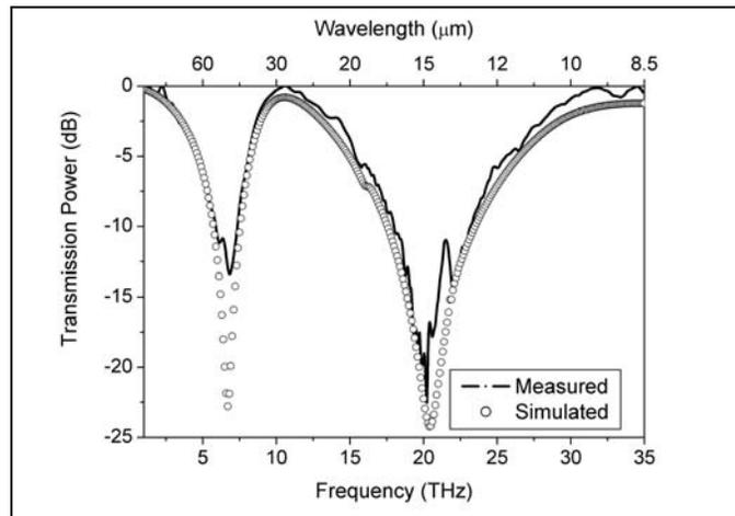
Comparison of the measured transmission spectrum for a fractal cross-dipole array to the response predicted by the PMM model with dielectric and metallic losses included. The measured stopbands are -13.4dB at 44μm and -22.5dB at 15μm.
